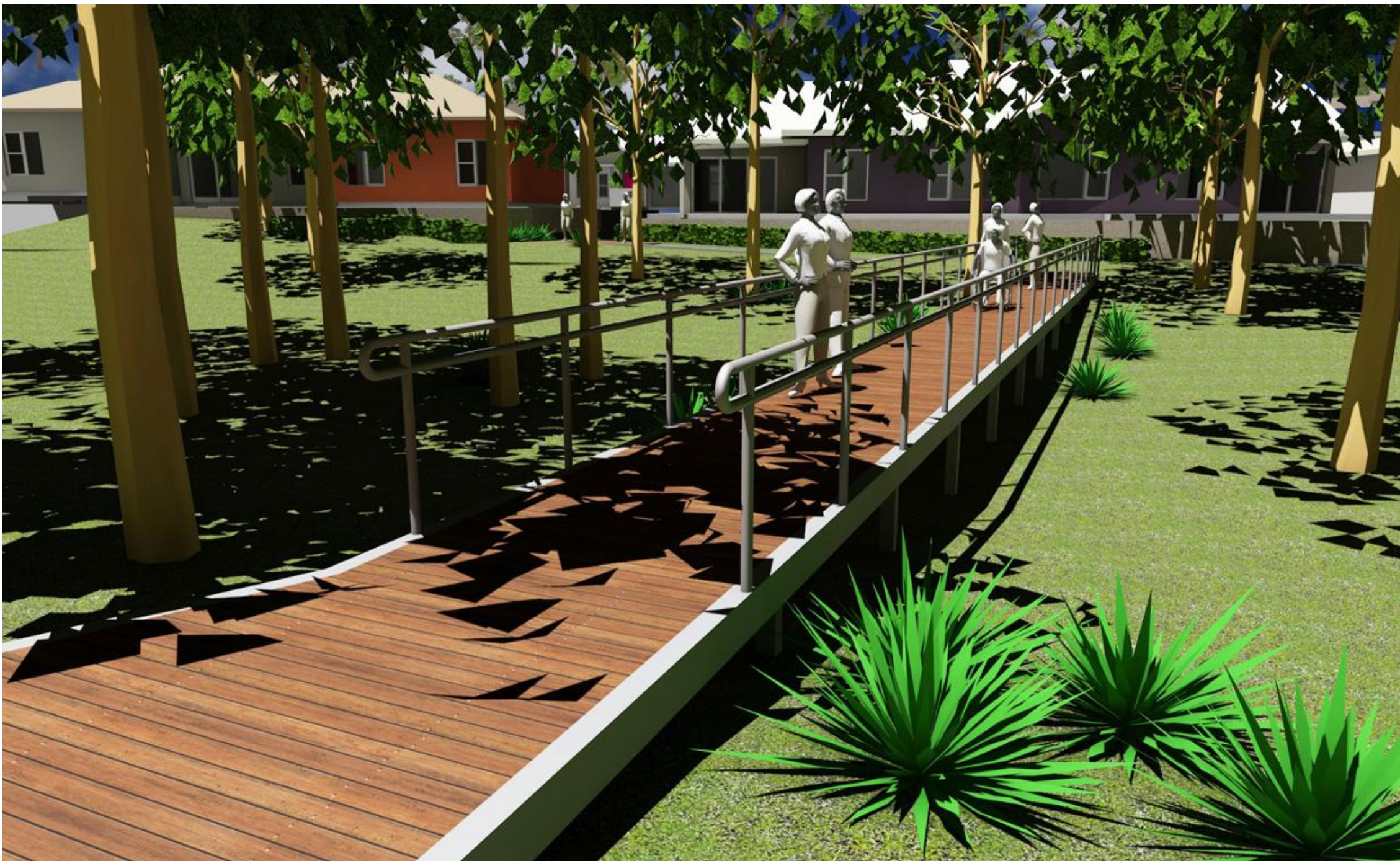
Illustrative image of pedestrian crossing over drainage easement - proposed as 1.8m wide timber [or timber composite] deck supported and edged with a galvanised steel structure and handrails where drop exceeds 0.5m (maximum height above natural ground 1.2-1.5m)
